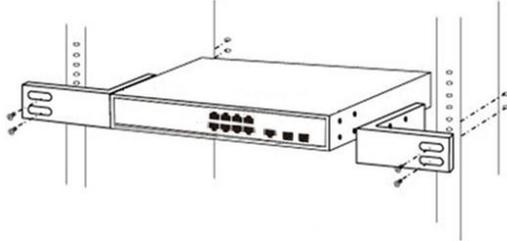
Step 4 Check and confirm the product is firmly installed on the rack, then mounting ends.
