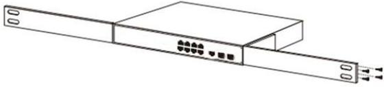
Step 3 Place the device into rack and adopt 4 screws to install the mounting lugs on the left and right side in the rack.
