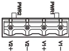
The device provides 4 pins power supply input terminal blocks and two independent DC power supply systems of PWR1 and PWR2. The power supply supports nonpolarity and anti-reverse connection. It can normally operate after reverse connection. Power supply range: 24VDC (12 ~ 48VDC)
