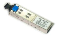
This mini-GBIC SFP Module is a plug-in device and it is hot-swappable. It allows for seamless integration between fiber and copper LAN connections wherever Gigabit SFP slots are available. This device is economical, saves time, offers flexibility and eliminates the need to replace ntire switches/converters/servers when customers need to change or upgrade fiber connections.
