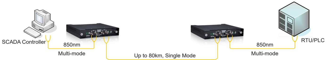
Typical Application Using TC3026 Fiber Optic Mode Converter
