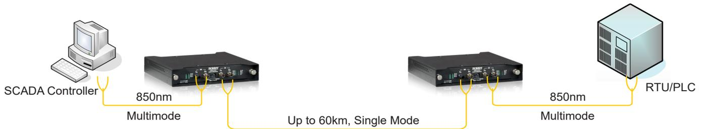
Typical Application Using TC3024 Fiber Optic Mode Converter
