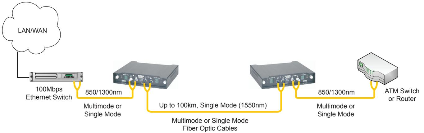
Typical applications using TC3004 Fiber Optic Mode Converter/Repeaters
