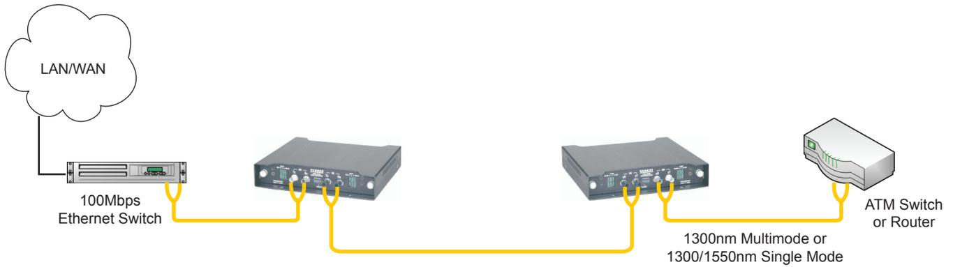
Typical applications using TC3004 Fiber Optic Mode Converter/Repeaters
