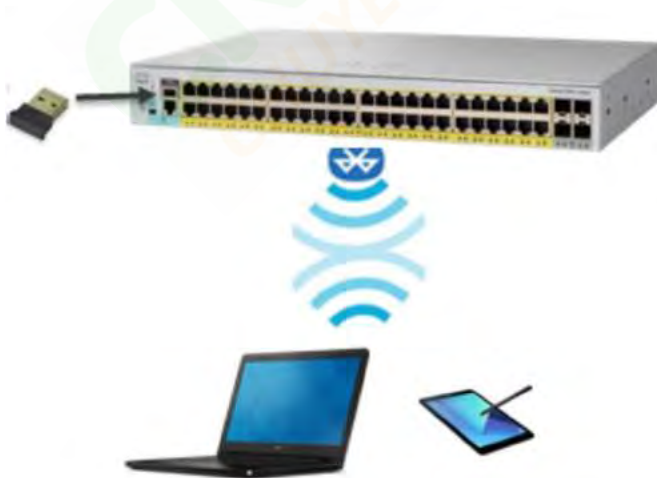
Figure 4. Over-the-air switch access using Bluetooth
