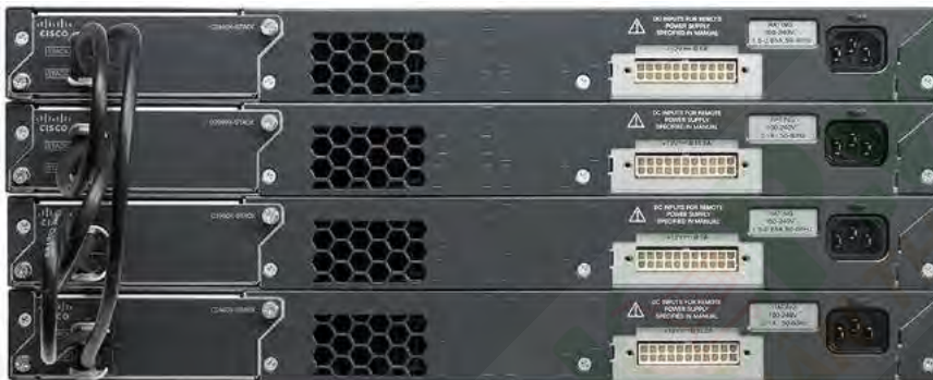
Figure 5. Cisco FlexStack-Plus switch stack
